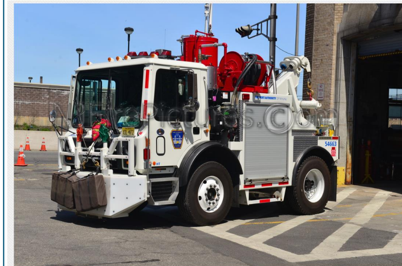
HOLLAND TUNNEL 54663 2015 MACK MRU/MILLER INDUSTRIES/ANSUL 50AFFF/150 PKP
